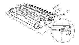
8 Install the drum unit and toner cartridge assembly in the machine.
