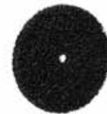
Scotch-Brite™ Clean and Strip Disc is designed to effectively clean welds, remove rust and strip paint. Our extra coarse grade open web discs provide a smooth running loading-resistant wheel, which is ideal for removing soft coatings.
