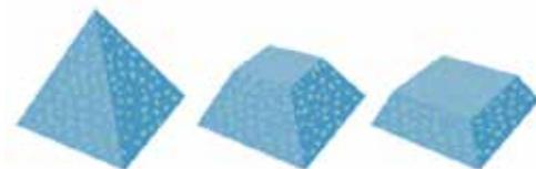
The three-dimensional structures of 3M™ Trizact™ Abrasives contain multiple layers of mineral. As these structures wear, fresh, sharp mineral is constantly exposed to the workpiece, resulting in faster, more consistent cutting throughout the life of the belt.
