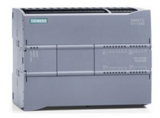
SIMATIC S7-1200, CPU 1215C, COMPACT CPU, AC/DC/RELAY, 2 PROFINET PORT, ONBOARD I/O: 14 DI 24V DC; 10 DO RELAY 2A, 2 AI 0-10V DC, 2 AO 0-20MA DC,
