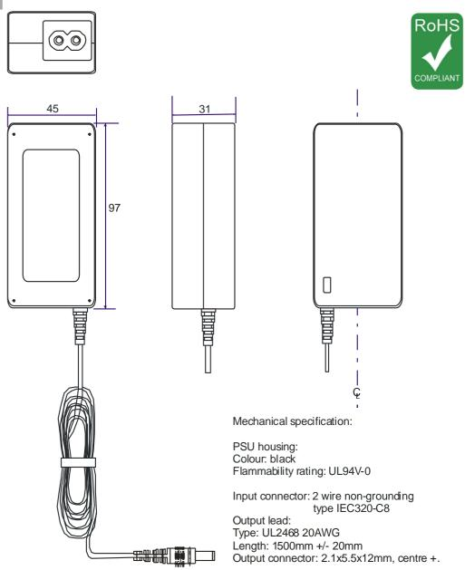
Mass: 0.145kg Tolerance on dimensions: +/- 0.5mm unless stated otherwise
