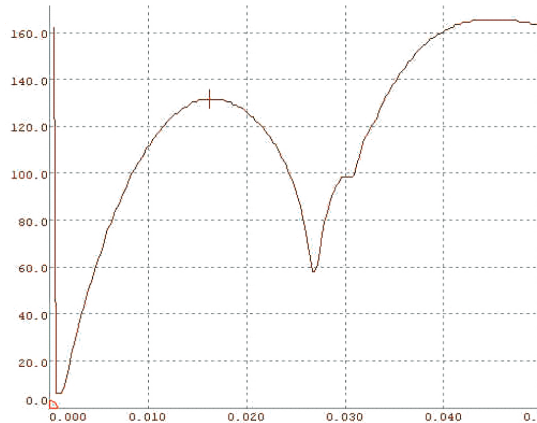
Figure 2: Search for the switching point with trace data from Automation Studio
