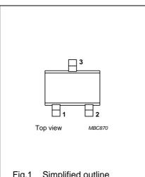
Fig.1 Simplified outline SOT323 and pin configuration.
