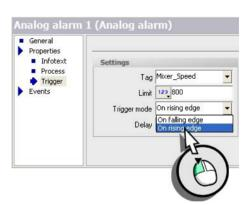
3. In the same way, configure the "Mixer speed too low" alarm. The alarm should be triggered when the speed drops below 400 (at "falling edge").
