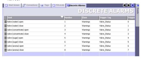
When you create the second discrete alarm by double-clicking on the empty line, the settings from the first discrete alarm are retained. The alarm number and bit number are automatically incremented.
