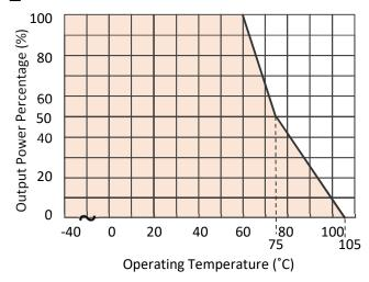
The derating curve was measured at nominal Vin in chamber with nature convection.
