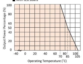
The derating curve was measured with nominal line. Mounted test board (90 x 80 mm and each power pin with 43 x 40 mm, 2Oz double layer)
