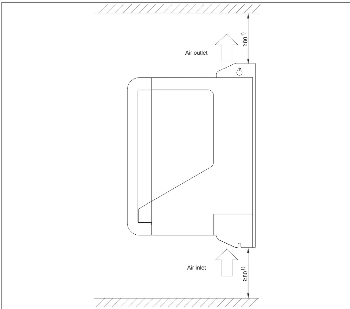
Figure 3: ACOPOS P3 8EI servo drives - Installation dimensions
