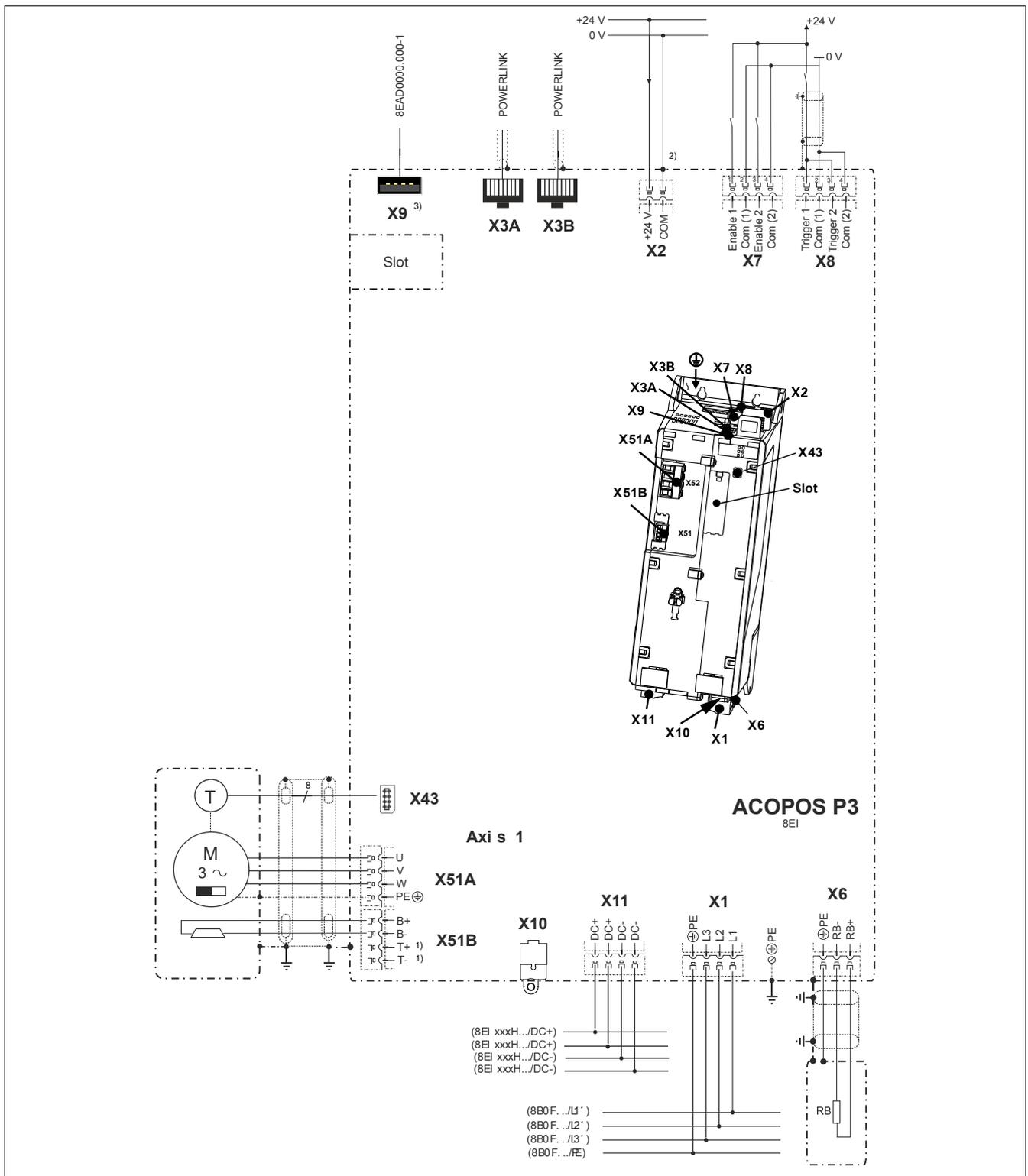
Figure 4: Mains input voltage - 3x 200 to 480 VAC
