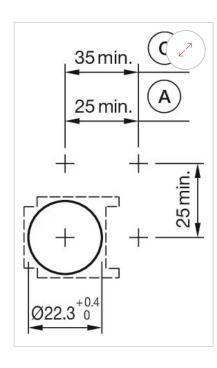
A = Solder/Plug-in terminal 2.8 mm x 0.5 mm
