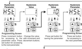
If no operation is performed in programming mode for 20 seconds, device turns to main operation screen automatically.
