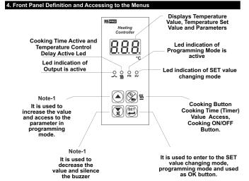
Note-1: If increment or decrement button is pressed for 5 seconds continuously, increment and decrement number become 10, if increment or decrement button is pressed for 10 seconds continuously, increment and decrement number become 100.
