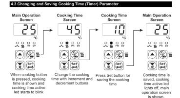
If no operation is performed in cooking time enter mode and set value enter mode for 20 seconds, device turns to main operation screen automatically.
