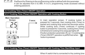
In main operation screen, If cooking button is pressed for 3 seconds, then cooking time (Timer) is started and cooking time active led becomes active. While cooking time (Timer) continues if cooking button is pressed for 3 seconds, cooking time (Timer) is finished and cooking time active led lights off. If button protection parameter PrE = 4 cooking time (Timer) ON/OFF operation is performed when button is pressed.
