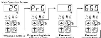
pressed for 5 seconds. PR" led starts to blink If programming mode button for accessing entering password is different from 0, programming mode entering screen
