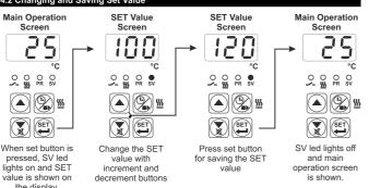
SET value changes according to maximum and minimum value of device type and scale. It can be adjusted from set value minimum parameter 5 ut value to set value maximum parameter
