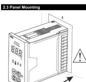
1-Before mounting the device in your panel, make sure that the cut-out is of the right size
