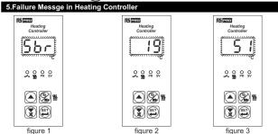
1- Probe failure in analog inputs. Sensor connection is wrong or there is no sensor connection When this message is on the screen, if buzzer function selection parameter  $\lceil \frac{1}{2} \rceil \Gamma \rceil$  is 3 or 4, internal buzzer starts to operate. See figure 1.
