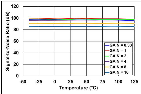
**FIGURE 2-31:** SNR vs. Temperature, Internal  $V_{REF}$ .
