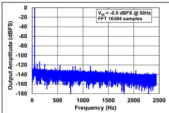
**FIGURE 2-3:** FFT Output Spectrum,  $f_{in} = 50 Hz$  (Internal  $V_{REF}$ ).
