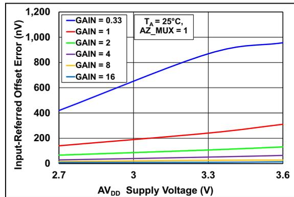
**FIGURE 2-47:** Offset Error vs.  $AV_{DD}$  ( $AZ\_MUX = 1$ ).
