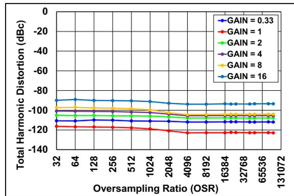
**FIGURE 2-12:** THD vs. OSR External  $V_{REF}$ .
