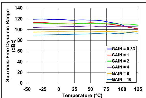
**FIGURE 2-33:** SFDR vs. Temperature, Internal  $V_{REF}$ .
