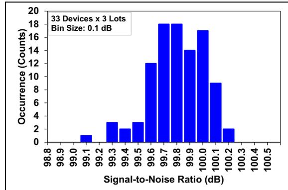
**FIGURE 2-22:** SNR Distribution Histogram Internal  $V_{REF}$ .
