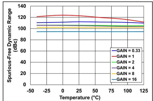
**FIGURE 2-29:** SFDR vs. Temperature, External  $V_{REF}$ .
