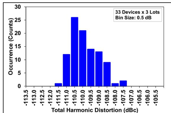
**FIGURE 2-24:** THD Distribution Histogram Internal  $V_{REF}$ .
