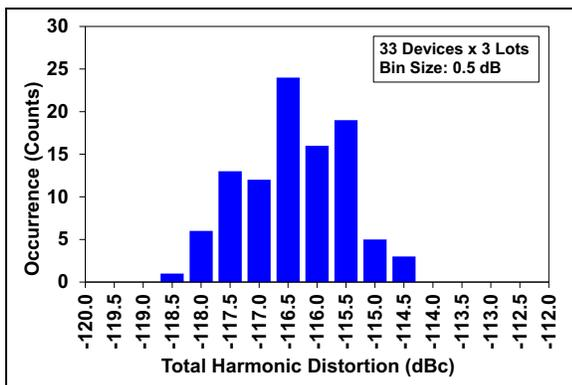
**FIGURE 2-20:** THD Distribution Histogram External  $V_{REF}$ .
