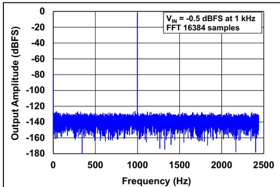
**FIGURE 2-2:** FFT Output Spectrum,  $f_{in} = 1 kHz$  (External  $V_{REF}$ ).
