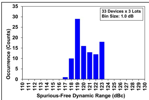
**FIGURE 2-21:** SFDR Distribution Histogram External  $V_{REF}$ .
