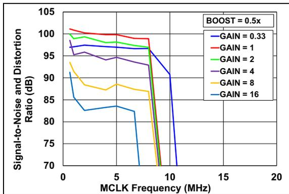
**FIGURE 2-39:** SINAD vs. AMCLK (BOOST = 0.5X, Internal  $V_{REF}$ ).
