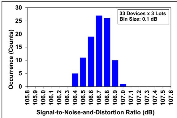
**FIGURE 2-19:** SINAD Distribution Histogram External  $V_{REF}$ .
