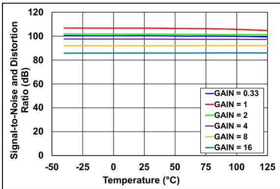
**FIGURE 2-26:** SINAD vs. Temperature, External  $V_{REF}$ .
