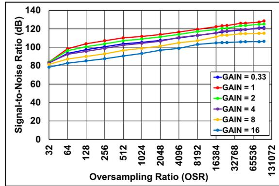
**FIGURE 2-11:** SNR vs. OSR External  $V_{REF}$ .
