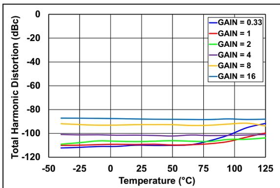
**FIGURE 2-32:** THD vs. Temperature, Internal  $V_{REF}$ .
