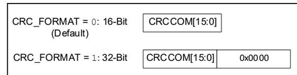
**FIGURE 6-10:** CRC Format Table for Read Communications.
