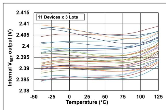
**FIGURE 2-59:**  $V_{REF}$  Output Voltage vs Temperature ( $AV_{DD} = 3.3V$ ).
