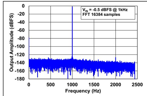
**FIGURE 2-4:** FFT Output Spectrum,  $f_{in} = 1 kHz$  (Internal  $V_{REF}$ ).
