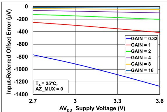
**FIGURE 2-45:** Offset Error vs.  $AV_{DD}$  ( $AZ\_MUX = 0$ ).
