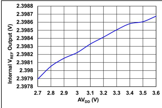
**FIGURE 2-60:** Internal  $V_{REF}$  Output Voltage vs.  $AV_{DD}$ .
