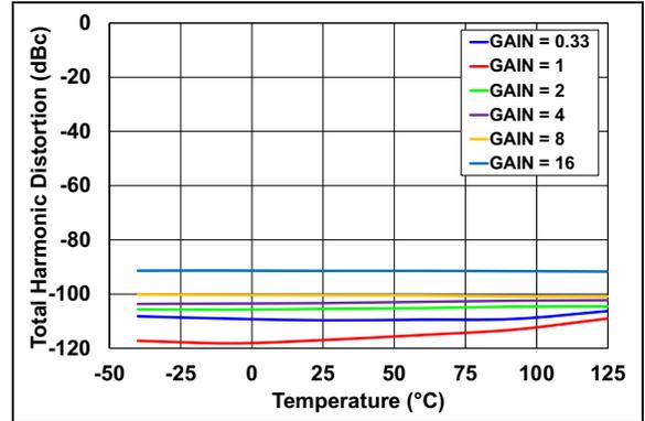
**FIGURE 2-28:** THD vs. Temperature, External  $V_{REF}$ .
