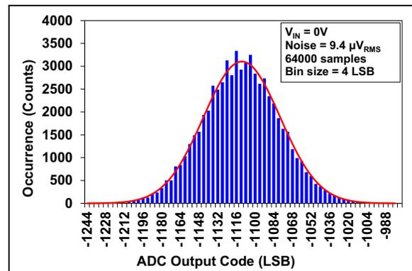
**FIGURE 2-6:** Output Noise Histogram (Internal  $V_{REF}$ ).
