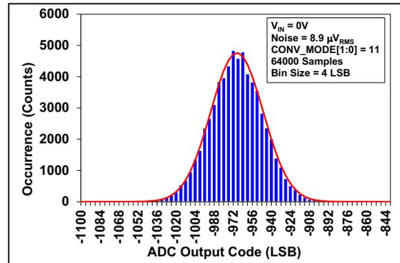
**FIGURE 2-5:** Output Noise Histogram (External  $V_{REF}$ ).
