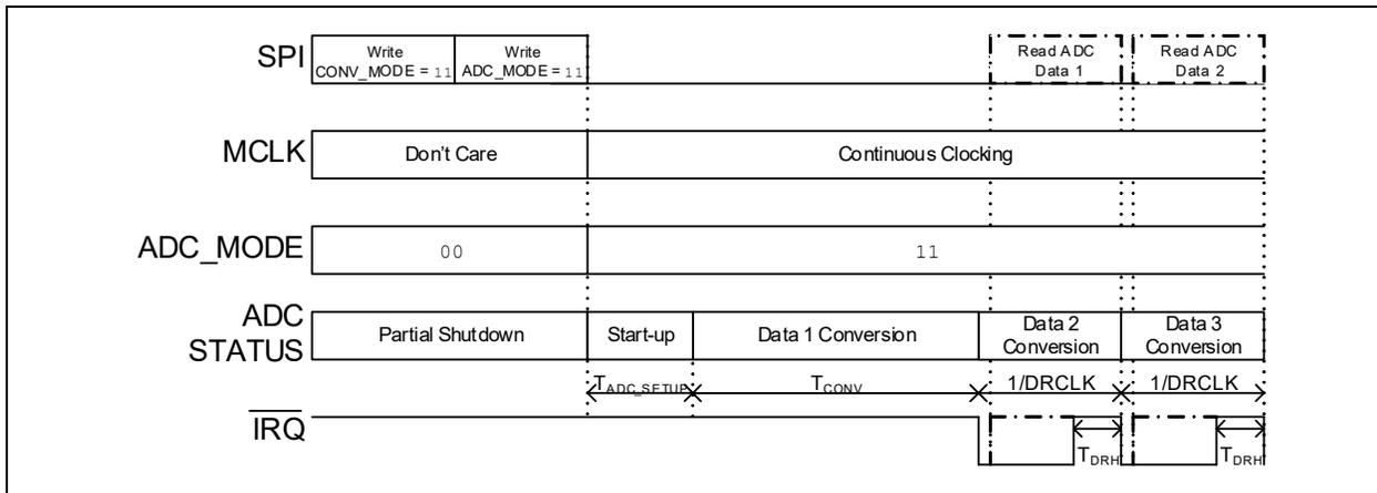
**FIGURE 5-15:** MUX Continuous Conversion Mode Timing Diagram.
