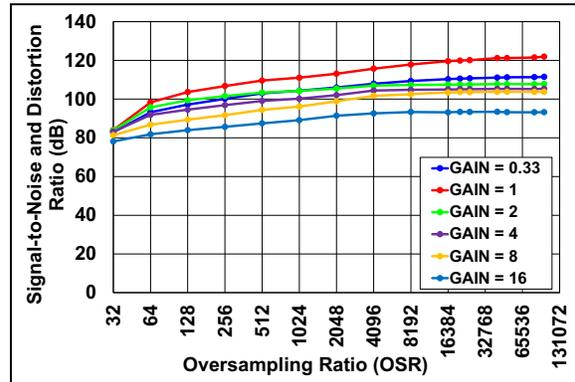
**FIGURE 2-10:** SINAD vs. OSR External  $V_{REF}$ .
