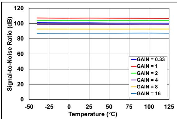
**FIGURE 2-27:** SNR vs. Temperature, External  $V_{REF}$ .
