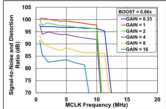
**FIGURE 2-40:** SINAD vs. AMCLK (BOOST = 0.66X, Internal  $V_{REF}$ ).
