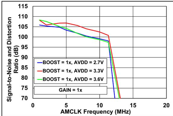
**FIGURE 2-43:** SINAD vs. AMCLK vs.  $AV_{DD}$ .
