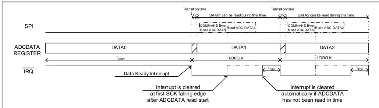
**FIGURE 6-13:** Data Ready Interrupt  $\overline{\text{IRQ}}$  Pin Timing Diagram.
