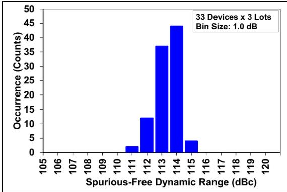
**FIGURE 2-25:** SFDR Distribution Histogram Internal  $V_{REF}$ .
