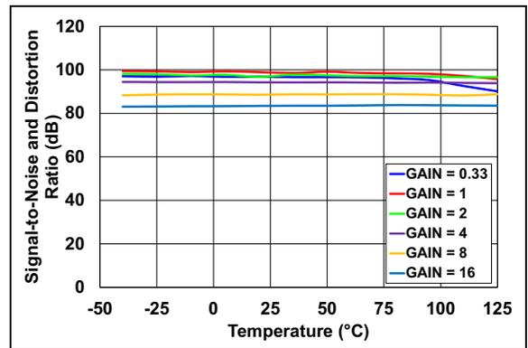
**FIGURE 2-30:** SINAD vs. Temperature, Internal  $V_{REF}$ .
