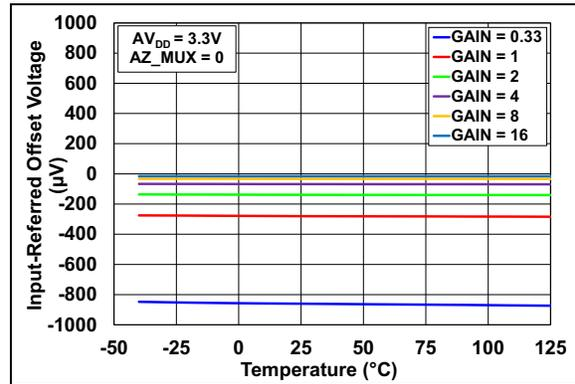
**FIGURE 2-46:** Offset Error vs. Temperature ( $AZ\_MUX = 0$ ).
