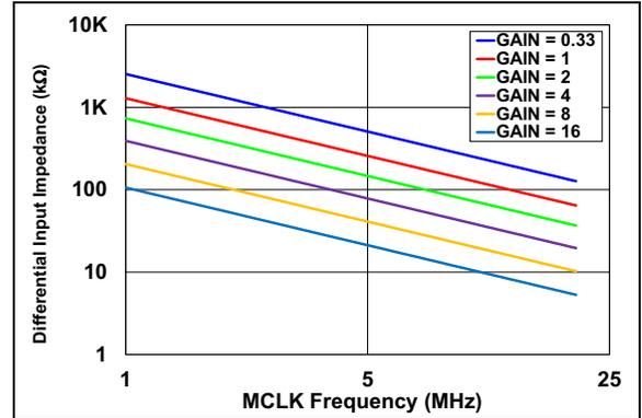
**FIGURE 2-52:** Differential Input Impedance vs.  $MCLK$ .
