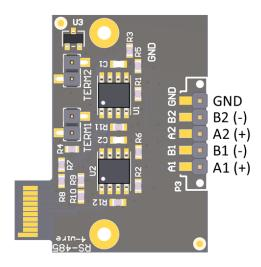
Termination Resistor Jumper for A1/B1
