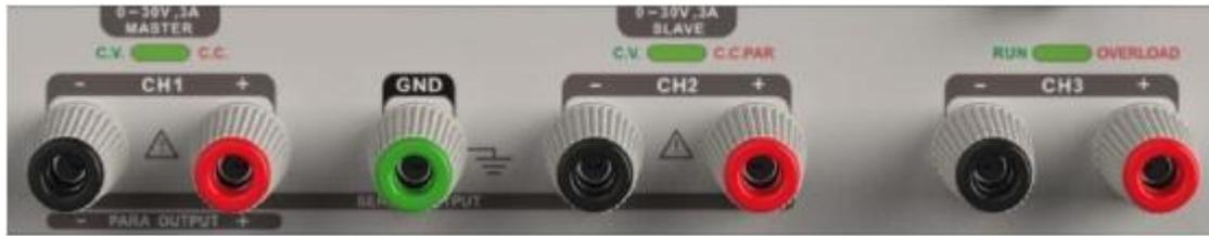
The positive/negative output terminals of CH1, CH2, CH3, and the common GND for CH1, CH2 are located on the front panel. Refer to later “control panel operation” for wiring method details.
