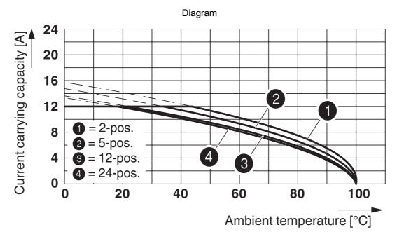
Type: ICC 2,5/...-ST-5,08 with IC 2,5/...-G-5,08; contact: ICC-MT 1,5 - 2,5
