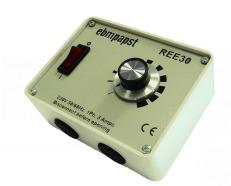
This single phase electronic control device provides a simple solution to speed controlling single or multiple fans. It has a manual dial which can change the fan speed from a minimum setting (factory set to approx 20%) to 100%.
