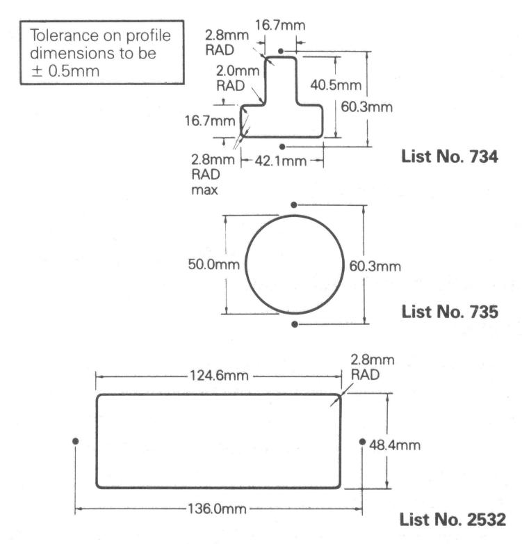
The panel onto which the socket-outlets are mounted must extend a minimum of 10mm in each direction from the aperture. Maximum panel thickness 2mm
