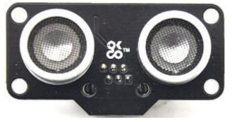
from the transmission to the reception, and then multiply the speed of the sound in the air(340 m/s) to calculate the distance from the sensor to the object.
