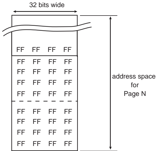
Step 1: Flash array after page erase
