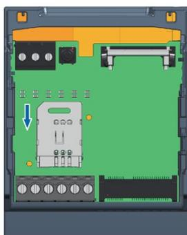
3. Put the SIM card in the card holder and then lock the card holder in the marked direction.
