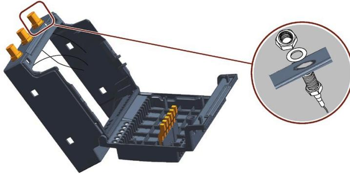
4. Install the middle housing back on the bottom housing. When install the middle housing, place the bottom of the SMA connectors below the top PCBA first, then adjust the position of the middle housing and install it back.
