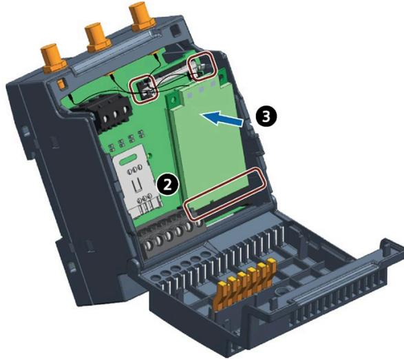
4. Connect the feeder cables with the corresponding antenna connectors of the cellular module. Arrange the feed lines and make them pass from the feeder cable path to prevent interruption.
