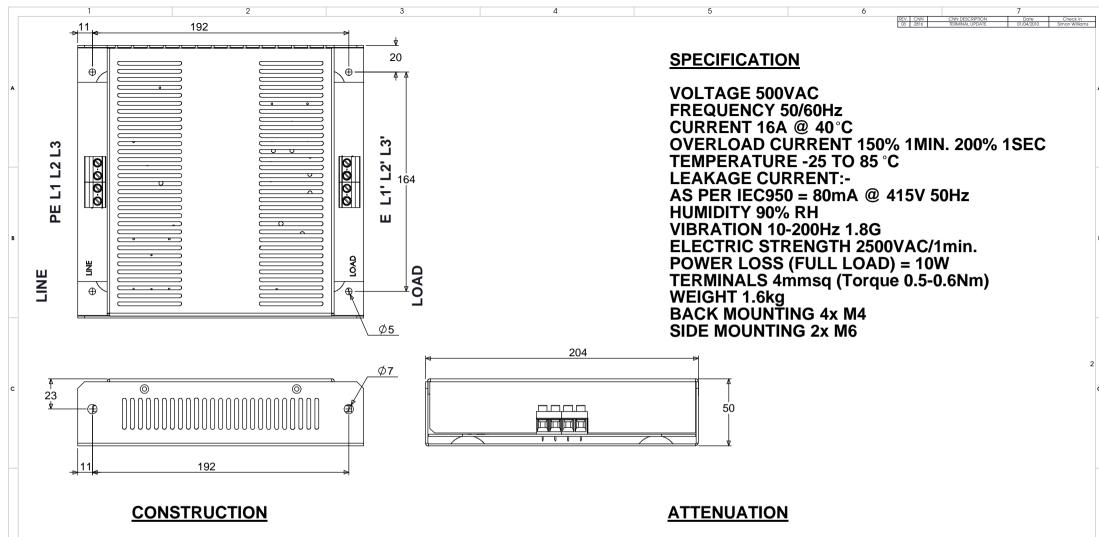
PERFORATED ALUMINIUM BODY FOR AIR COOLING, ALL COMPONENTS PCB MOUNTED
