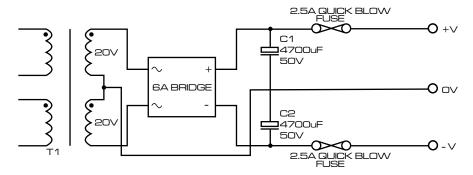
T1 = 50VA 20-0, 20-0 C1/C2 = 4700uF 50V ELECTROLYTICS BRIDGE = 6A 200V PIV THE MAINS INPUT PRIMARY MUST BE PROTECTED BY A HBC CERAMIC FUSE. A 2.5A RATING IS SUGGESTED.
