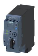
SIRIUS Compact load feeder DOL starter 690 V 24 V AC/DC 50...60 Hz 1...4 A IP20 Connection main circuit: plug-in, without terminals Connection auxiliary circuit: plug-in, without terminals
