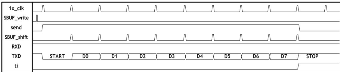
Figure 6.8 Timing Diagram for UART Transmission Mode1
