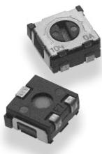
Consuming just 10.5 sq.mm of board, the 3203 has been developed specifically for a new generation of hand held equipment, where mixed technology and double sided component placement are unavoidable. These 3mm devices are just 2mm high and sealed for IR, vapour phase and full immersion wave soldering together with solvent board washing process. Also available within this range is the 3213, the auto adjust sister to the 3203.
