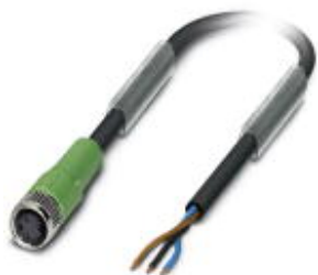
Sensor/Actuator cable, 3-position, PUR halogen-free, black-gray RAL 7021, free cable end, on Socket straight M8, Cable length: 5 m
