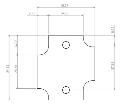
Dashed line shows outline of the mounting boss under PCB board Recommended mounting holes diameter ø3,5mm
