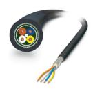
By the meter, Data cable, PROFINET CAT5 (100 Mbps), shielded, PE-X halogen-free, black RAL 9005, 4-wire (1x4xAWG22/7, SF/TQ), color single wire: white-blue, orange-yellow, cable length: Free input (0.5  $\dots$  100 m)
