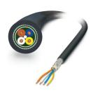
By the meter, Data cable, PROFINET CAT5 (100 Mbps), EtherCAT® CAT5 (100 Mbps), shielded, PE-X halogen-free, black RAL 9005, 4-wire (1x4xAWG22/7, SF/TQ), color single wire: white-blue, orange-yellow, cable length: Free entry (0. 5  $\dots$  400 m)
