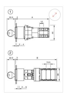
1 = Kraus & Naimer switching element A = (Number of stages x 12) + 66.5 mm 2 = Santon switching element B = (Number of stages x 13.5) + 65.5 mm
