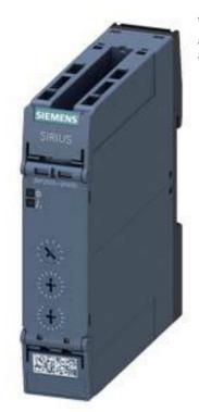
Timing relay, Multifunction 2 change-over contacts, 13 functions Positively driven Relay contacts 24...240 V AC/DC at 50/60 Hz AC 7 time ranges (0.05 s...100 h) with LED Spring-type terminal (push-in)
