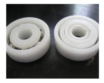
machined bearing began to wear much faster, generating more heat. After 1.5 hours and 90,000 revolutions the inner raceway of the machined plastic bearing melted and the bearing failed. BNL's bearing completed the test.
