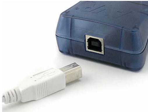
When the AVRISP mkII is connected to the PC, and if the USB driver is installed, the green LED inside the AVRISP mkII close to the USB connector will be lit. The main status LED will be red before target is detected.
