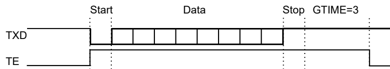
Figure 32-19. Example of TE Drive with Guard Time
