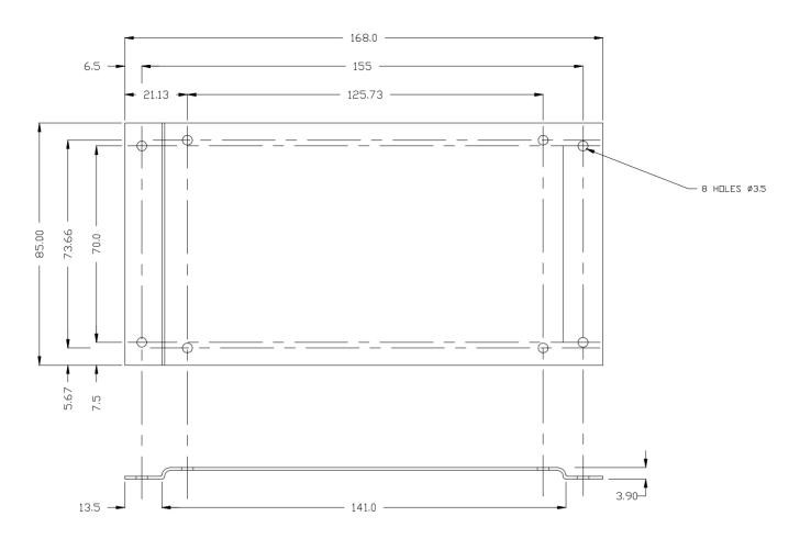
MATERIAL 1.0mm THICK MILD STEEL FINISH ZINC PLATE & COLDUR PASIVATE
