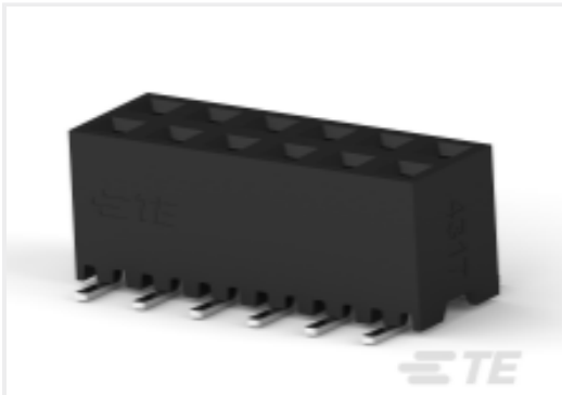
TE Part # 1-2314844-2 12P,2MM,B-B,REC,DRV,T,SMD,0.1AU,TB,W/CP
