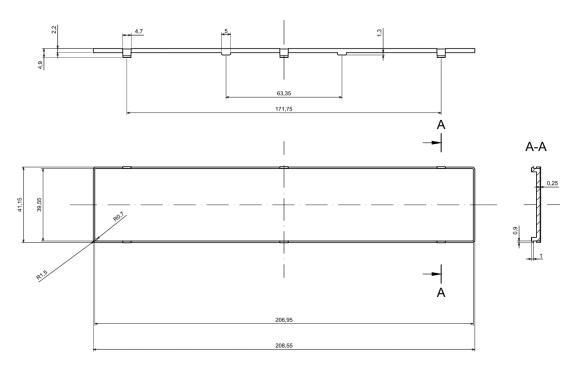
All dimensions are given within +/-0,5mm tolerance
