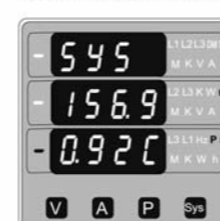
Screen 7 : System Phase Angle & power factor (3P4W & 3W)
