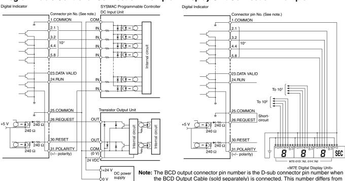
the BCD output connector pin number is the D-sub connector pin number when the BCD Output Cable (sold separately) is connected. This number differs from the pin number for the Digital Indicator narrow pitch connector (manufactured by Honda Tsushin Kogyo Co., Ltd.).
