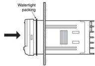
Insert the adapter into the grooves on the left and right sides of the rear case and push until it reaches the panel and is fixed in place.
