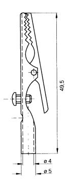
Crocodile clip with nickel-plated steel clamp. Can clamp pins up to 5 mm in diameter. 4 mm dia. socket connection plus connection via a locking screw. Solder connection is also possible.
