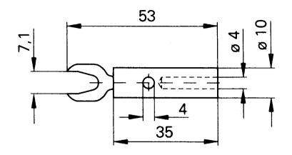
Cable lug with insulating sleeve, transverse hole and socket connection, diameter 4 mm. Fits on pins between 4 and 7 mm in diameter. Nickel-plated brass contact.
