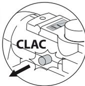
Protection by thermal circuit breaker
