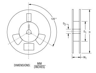
Devices are packed as shown here in compliance with EIA-481-C standard.
