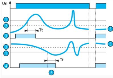
The under or overvoltage threshold value is set by a graduated potentiometer by reading the Un scale to be monitored directly. The hysteresis is set by a graduated potentiometer from 5 to 20 % of the preset threshold. The hysteresis value cannot be higher than the extremes of the measurement range. In overvoltage mode, if the controlled voltage exceeds the preset threshold for longer than the time set on the front face (0.1 to 10 s), the output relay opens and LED R is extinguished. During the
