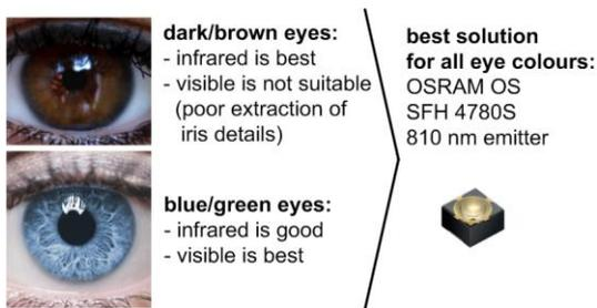
**Fig. 3:** Suitable wavelengths for iris scanning. 810 nm presents the best solution for all eye colors. Additionally the specular reflection of the corneal is low at 810 nm.
