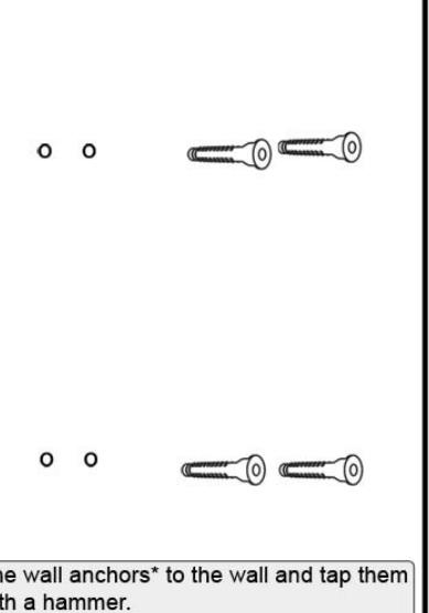
Insert the wall anchors\* to the wall and tap them flush with a hammer.
