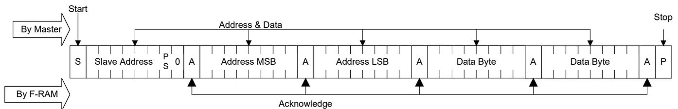
Figure 10. Hs-mode Byte Write
