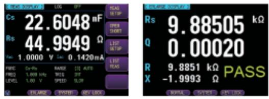
**MEAS Display** Parameter Setting and Four Measurement Parameters
