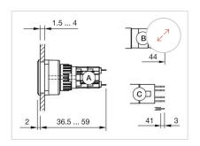
A = Solder terminal B = Plug-in terminal 2.8 mm x 0.5 mm C = Universal terminal 2.0 mm x 0.5 mm
