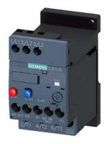
Overload relay 9.0...12.5 A Thermal For motor protection Size S00, Class 10 Stand-alone installation Main circuit: Screw Auxiliary circuit: Screw Manual-Automatic-Reset
