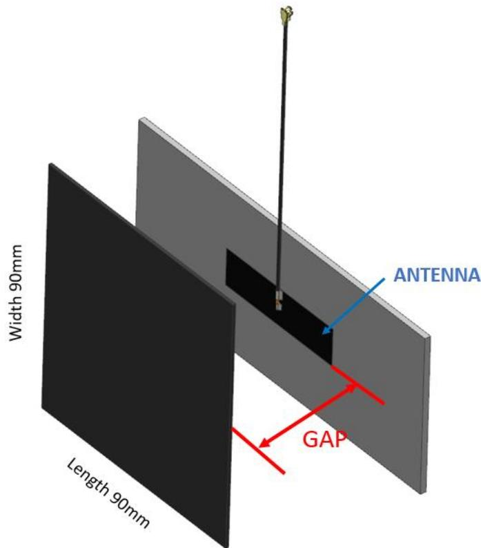
**FIGURE 6.1.1 FOUR LOCATIONS WITH PARALLEL PLANE GROUND**
