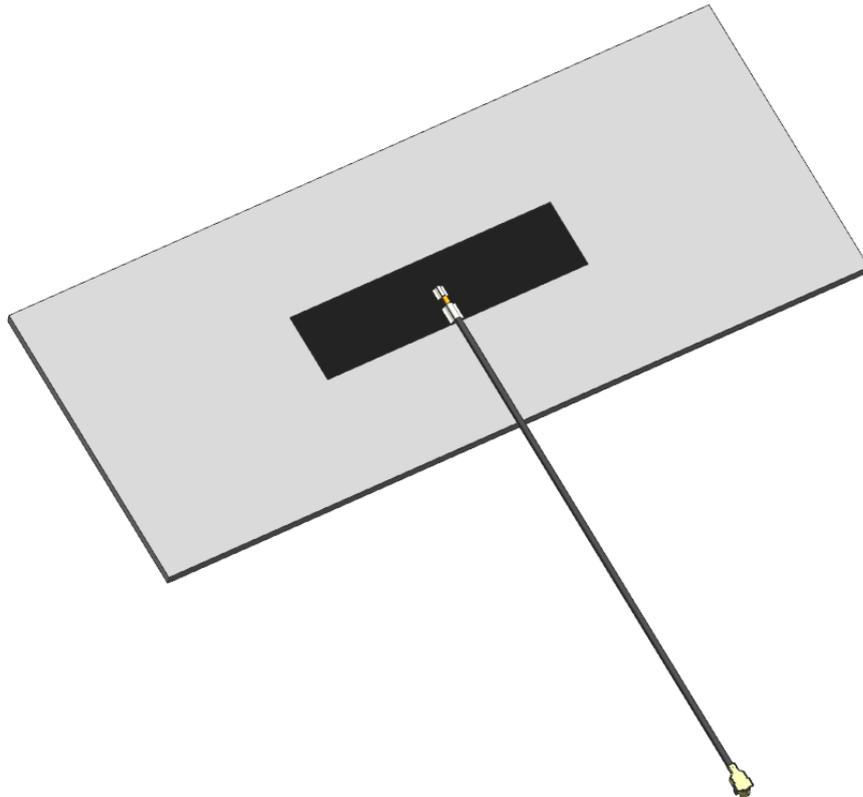
**FIGURE4.1.1 ANTENNA LOADED WITH PC/ABS BLOCK OF 1.5 MM THICKNESS**
