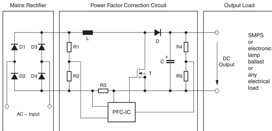
Fig. 4 - Typical Boost Converter Topology for Active PFC
